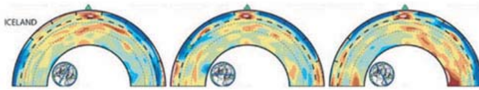
Figure 3. Global S-wave mantle tomography by J. Ritsema and coworkers (Model S20RTS: the so-called "Caltech model"). Cross sections beneath Iceland sliced at three different angles are shown [from Ritsema & Allen, 2003]. This model is derived from free-oscillation splitting, surface-wave dispersion, and body-wave traveltimes measurements.
