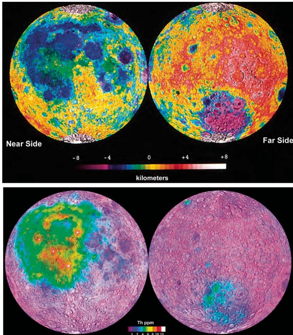
Figure 3. Top: Topography of front and back hemispheres of the Moon, illustrating saturation of the surface by impact structures between ca. 4.5 and 3.8 Ga. Bottom: Thorium content of surface materials. Diameter of the Moon is 3500 km. Clementine and Lunar Prospector maps provided by National Aeronautics and Space Administration.
