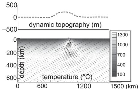
**Figure 2.** Dynamic uplift (upper panel) resulting from late synrift mantle flow (lower panel). Arrows are mantle flow lines, gray scale is temperature (in °C). Approximately 200 m maximum dynamic uplift is predicted centered on the rift.
