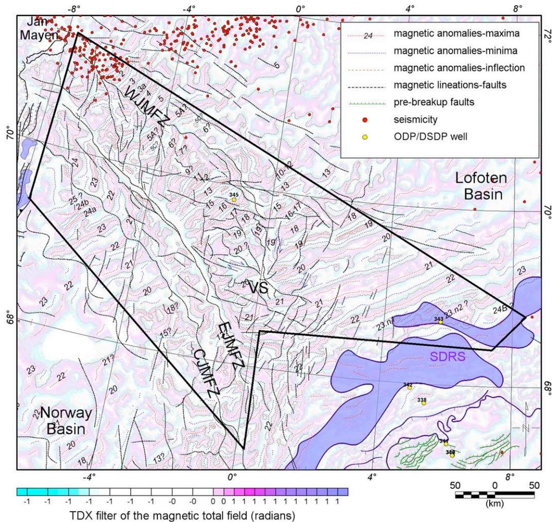
**Fig. 6.** TDX filter of the magnetic total field and overlying interpretation of the magnetic anomalies. The dashed lines represent maximum, minima and inflection points detected for each magnetic anomaly. The map also shows the main magnetic lineaments and chrons have been interpreted with reference to the chronostratigraphic time scale of [Cande and Kent, \(1995\)](#). VS: Vøring Spur.
