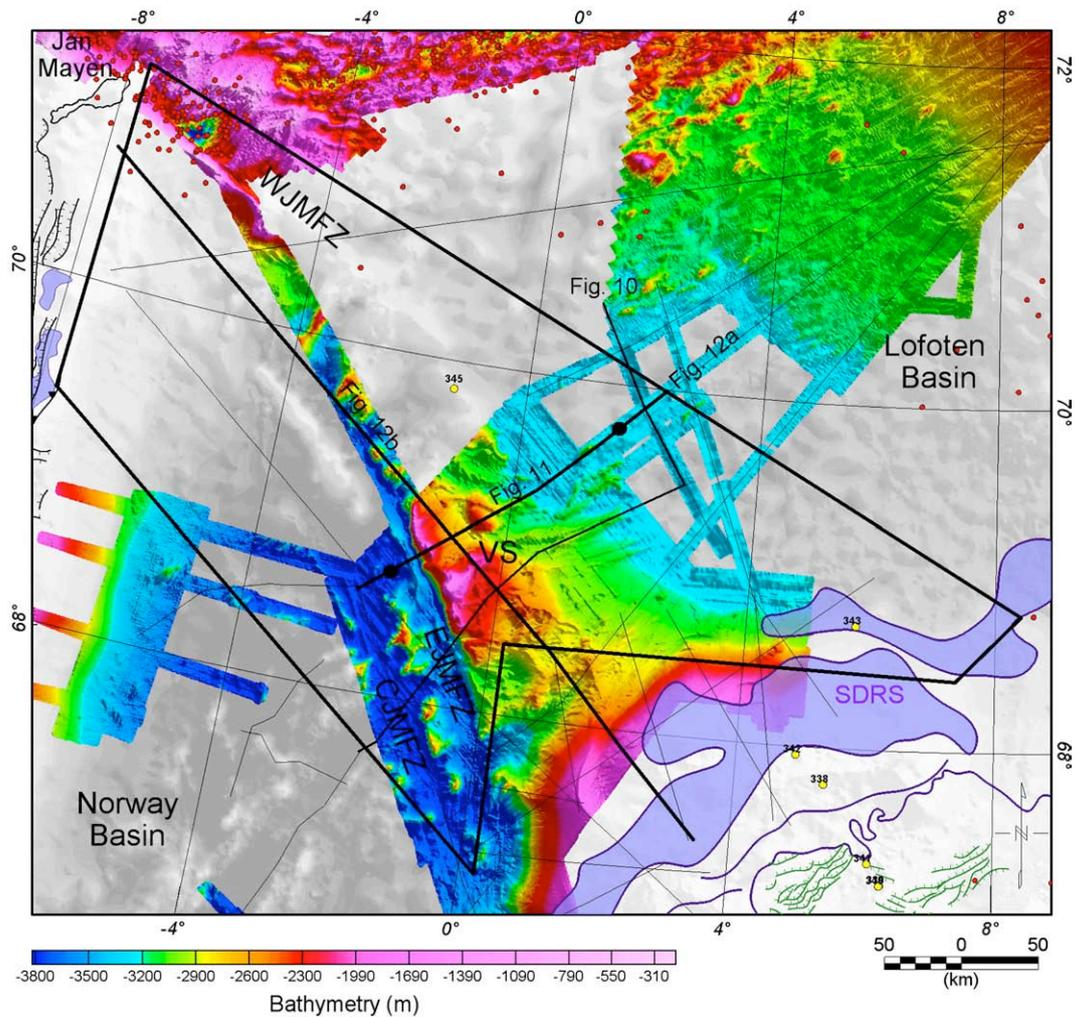
**Fig. 5.** High resolution bathymetric data merged with bathymetry derived from satellite altimetry (grey background) along the JAS-05 survey area. The Vøring Spur (VS) represents an atypical bathymetric high, located west of the Vøring Marginal High. VS: Vøring Spur.
