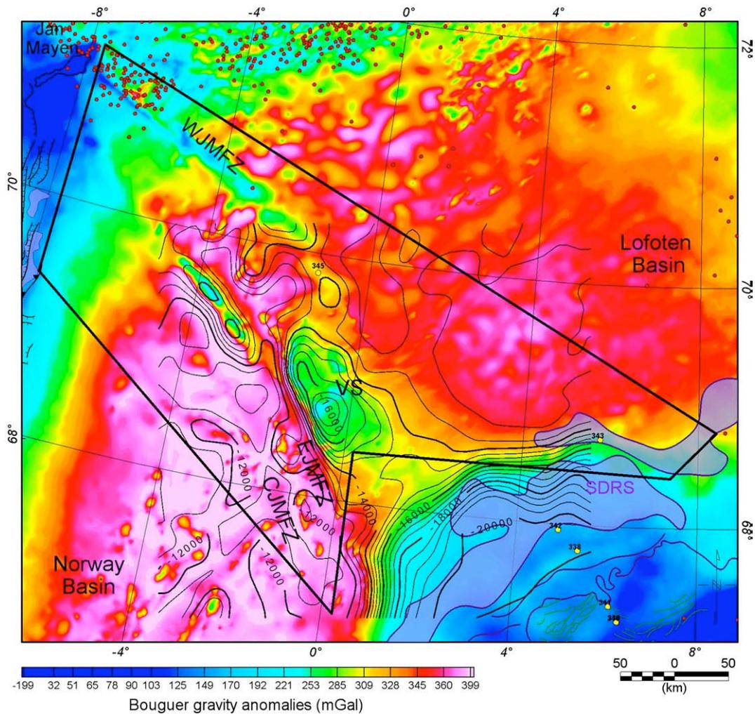
**Fig. 8.** Bouguer anomalies map combined with depth contours of the flexural Moho estimated for low elastic thickness ( $T_e = 1$  km). The Vøring Spur (VS) is characterised by an apparent Bouguer low, contrasting with the surrounding oceanic domains. The gravity low coincides with a thick oceanic crust ( $> 15$  km) between the Lofoten and Norway Basins.
