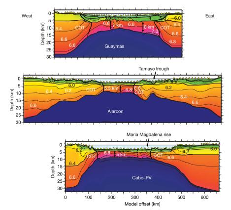
Figure 2 | Models of seismic velocity structure along the Guaymas, Alarcón and the San José del Cabo to Puerto Vallarta transects of the PESCADOR experiment. Velocity contours are colour-coded and labelled in units of  $\rm km\,s^{-1}$ . Yellow diamonds are the instrument locations. COT indicates the interpreted continent/ocean transition. The dashed line in the Cabo–PV
