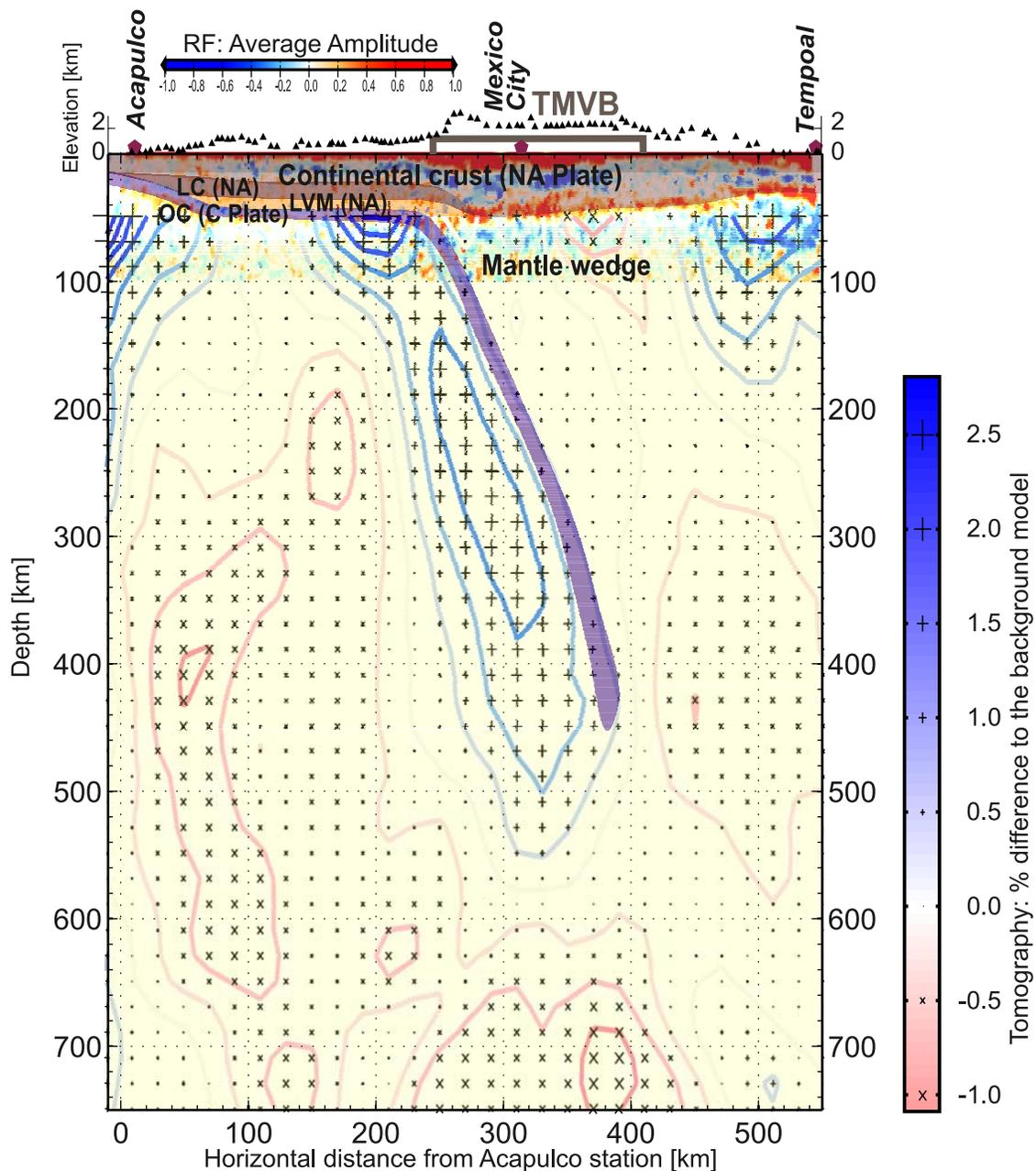
**Figure 3.** Composite model: tomographic and RF image showing the flat and descending segments of the slab. The key features are the flat under-plated subduction for 250 km, and the location and truncation of the slab at 500 km. The zone separating the ocean crust from the continental Moho is estimated to be less than 10 km in thickness. NA = North America, C = Cocos, LC = lower crust, LVM = low velocity mantle, OC = oceanic crust.
