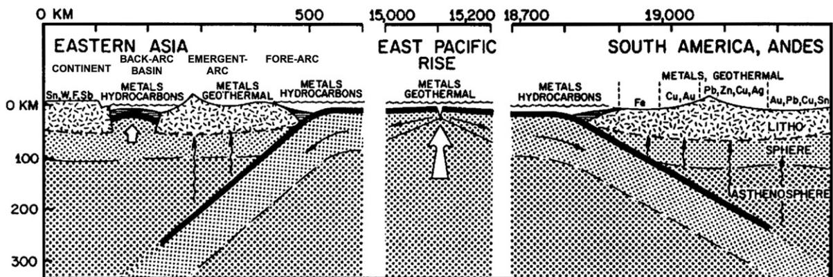
Fig. 10. Diagrammatic east–west cross-section of the Pacific Ocean between South America and southeast Asia showing settings for hydrothermal mineralization associated with convergent (subduction zones) and divergent (ocean ridges) plate boundaries and metallogenic zones of the Andes (modified from Rona, 1983b; Sillitoe and Perello, 2005).
