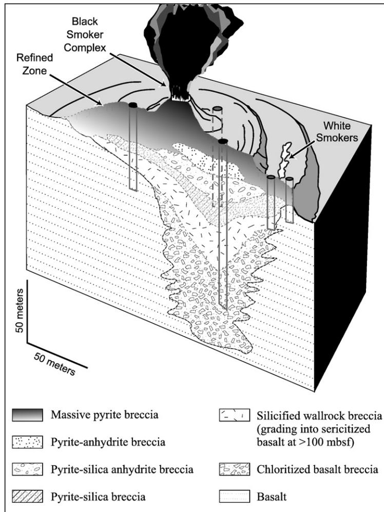
Fig. 9. Schematic cross-section through the TAG active massive sulfide mound (Fig. 8) showing characteristic surface and sub-surface features of a seafloor VMS deposit based on results of Ocean Drilling Program Leg 158 (Rona, 1992; Hannington et al., 1995; Humphris et al., 1995a,b).
