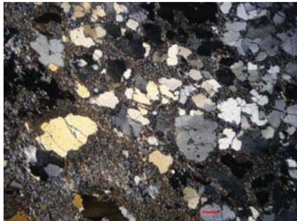
Figure 4a: Poorly sorted and texturally immature Dhanjori sandstone (red bar length 0.2 mm). Note the dominance of angular quartz and rock fragments.
