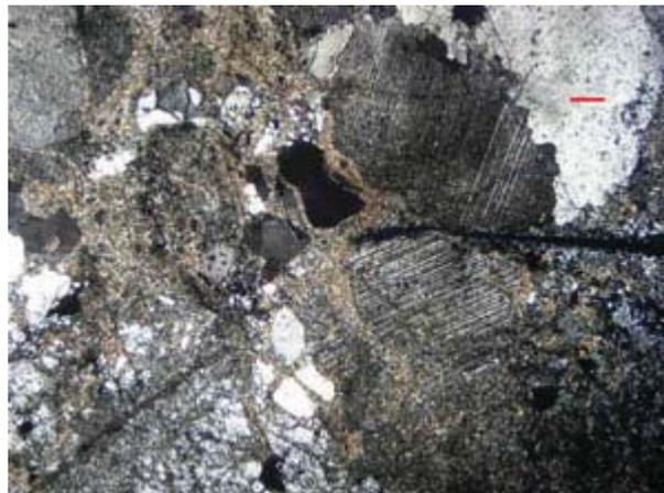
Figure 4b: Coarse-grained, feldspar-rich Dhanjori sandstone (red bar length 0.2 mm).
