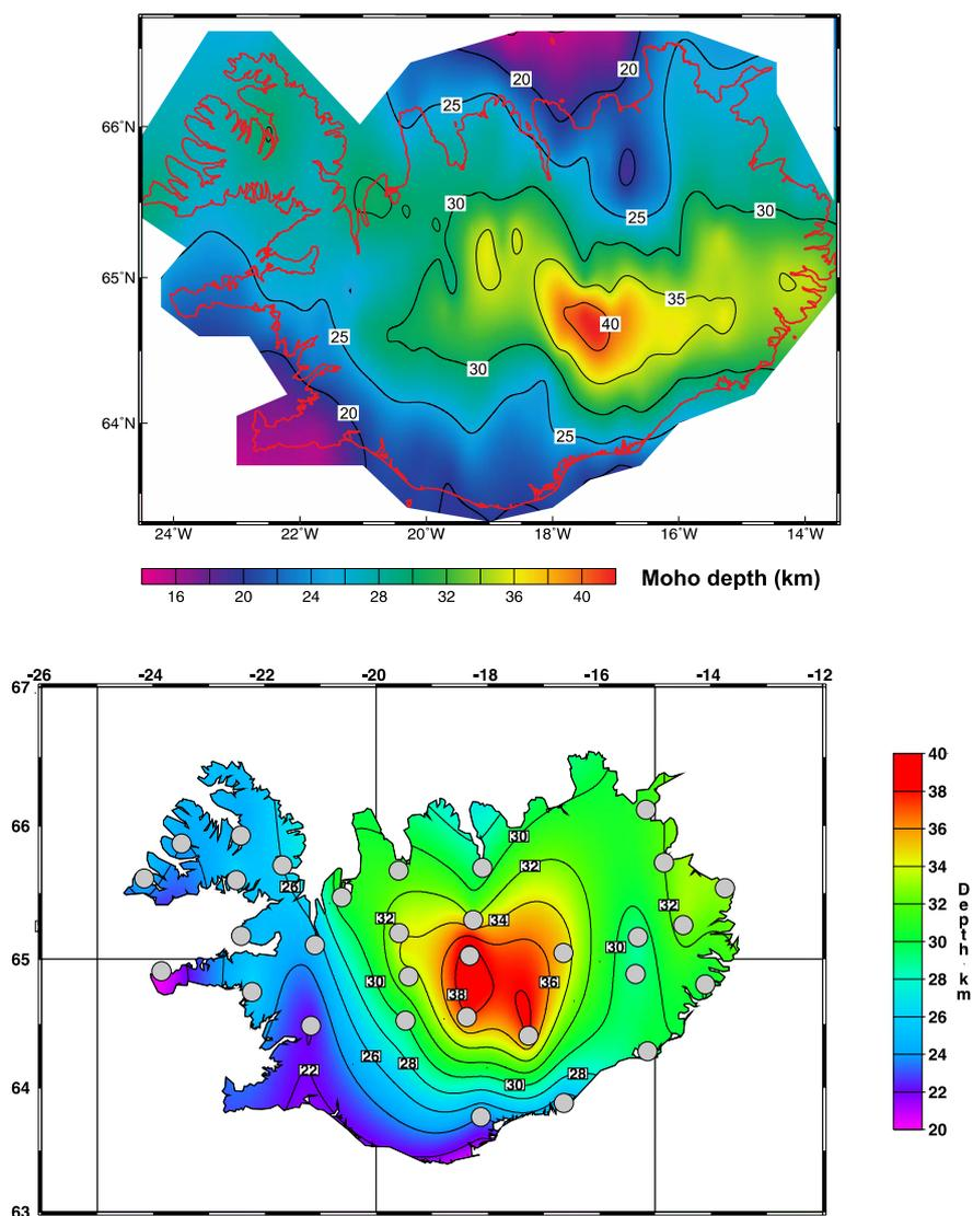
Figure 1: Top: Contour map of total crustal thickness determined using a combination of seismic profiles, receiver functions and gravity profiles [from Darbyshire et al., 1998]. Bottom: the lower crust defined as the depth to the  $V_s = 4.1 \text{ km s}^{-1}$  horizon [from Foulger et al., 2003].
