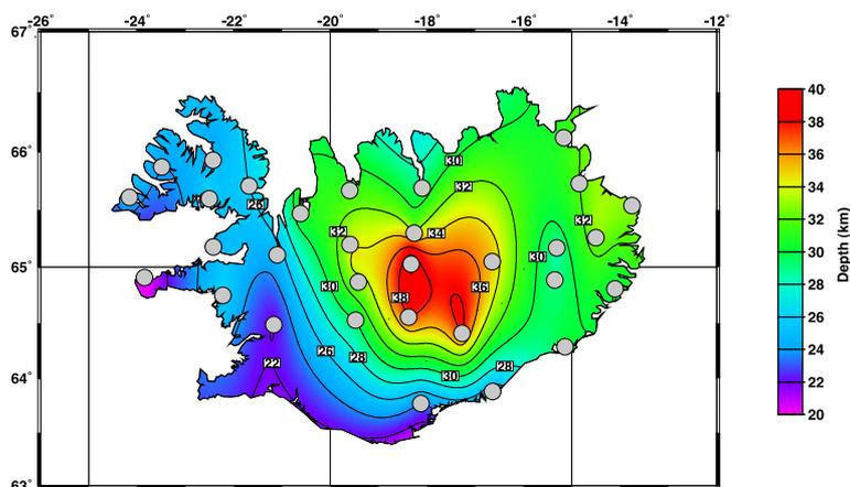
Figure 4: Contour map showing the depth to the base of the  $V_s = 3.7$  km/s horizon, approximately equivalent to the top of Layer 4, from seismic receiver functions. Gray circles indicate seismic stations [from Foulger & Anderson, 2005; Foulger *et al.*, 2003].
