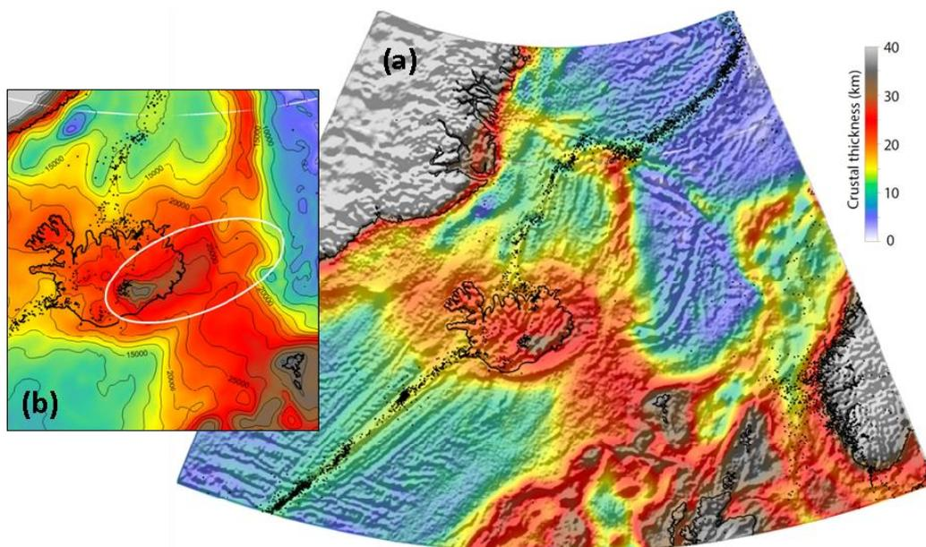
Figure 1 (a) Present day crustal thickness from gravity inversion for the NE Atlantic Ocean. (b) Higher resolution map of crustal thickness for E Iceland.
