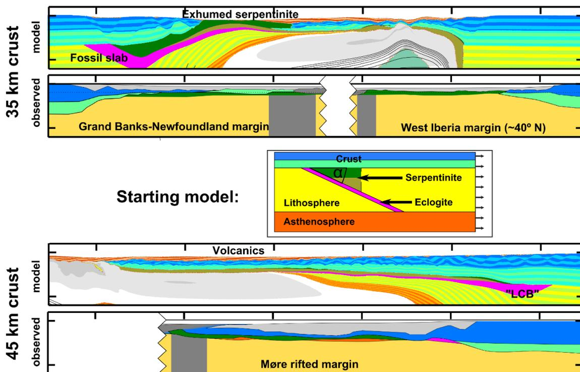
Figure 1: The starting model (middle panel) has three variable parameters, which are tested during the numerical simulations (crustal thickness, dip angle of the fossil eclogite slab and the rate of extension). Two results from the numerical simulations and possible observed analogues for a 35 km thick crust (upper panel) and 45 km thick crust (lower panel), could act as end member models for a magma-poor or magma-rich passive margin type, respectively.
