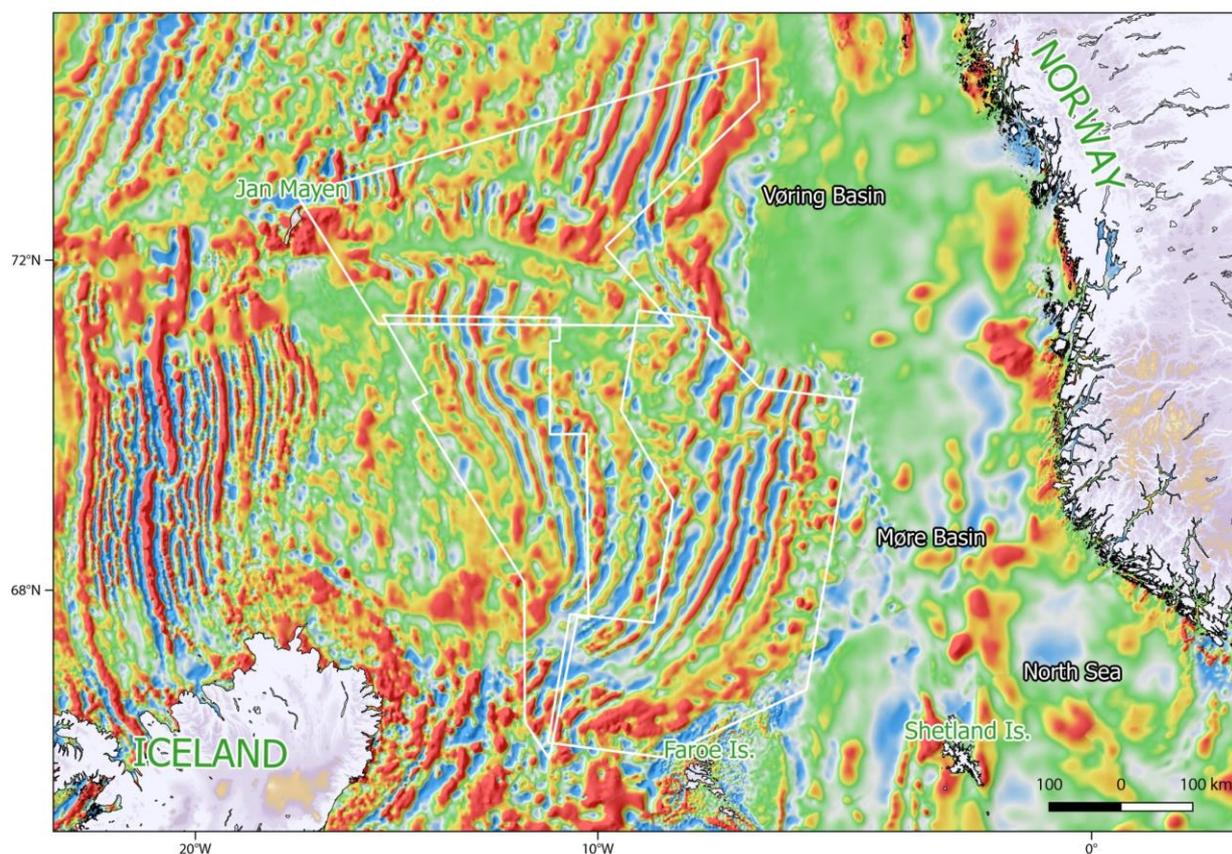
**Figure 4:** *New regional magnetic compilation of the Norway Basin. A total of ~88000 km of new magnetic profiles greatly improve the magnetic coverage of the Norway Basin and surrounding volcanic rifted margins. Details of the new surveys (white polygons) are further documented in Gernigon et al. (2015).*
