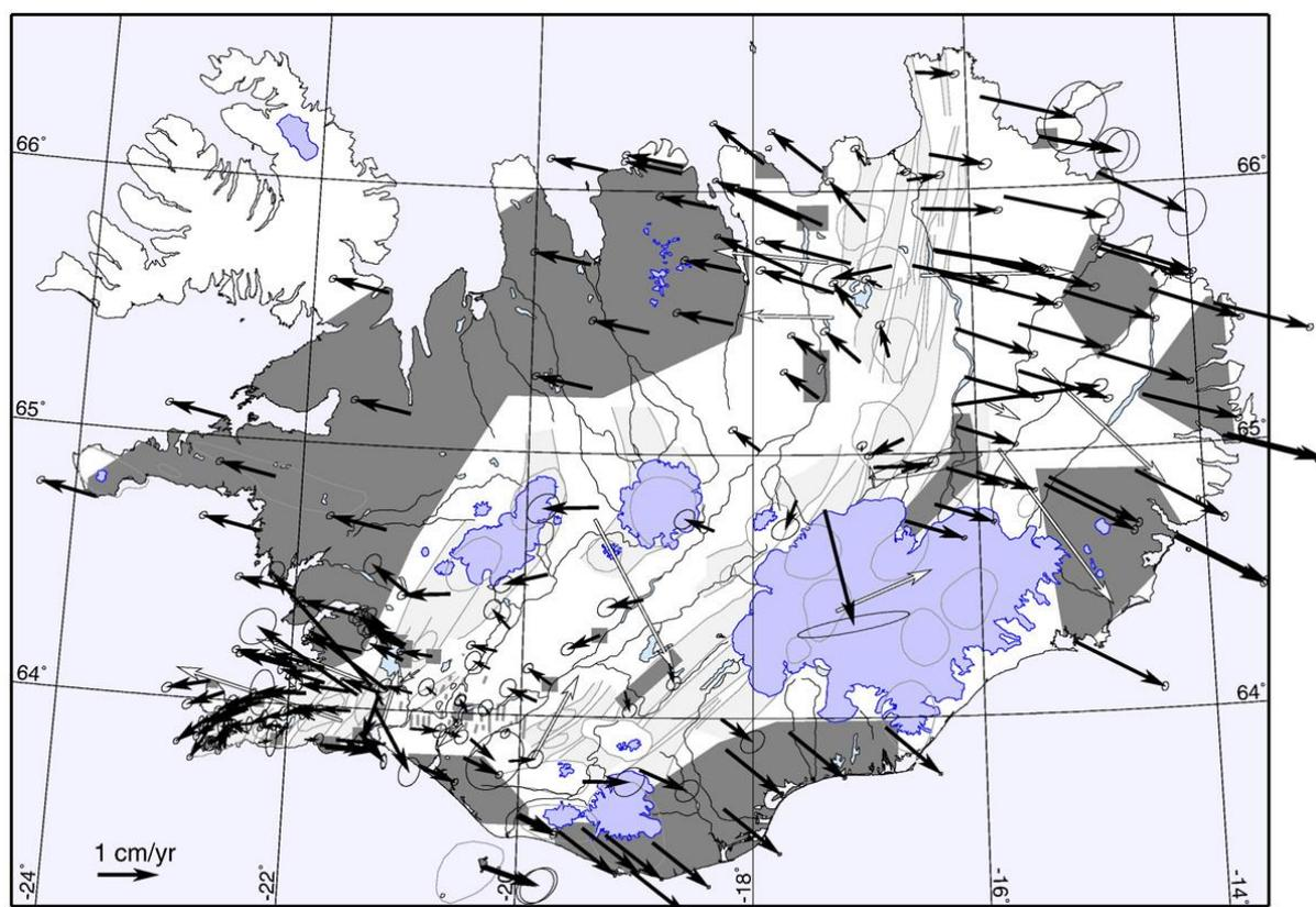
*Figure 7: Vectors of horizontal velocity from GPS data between 1986 and 2002 with  $1\sigma$  standard deviations. Blue: icecaps, dark grey: blocks considered by Perlt et al. [2008] to be tectonically inactive. However, it is likely that no part of Iceland is truly inactive. Insignificant velocity vectors are not filled [reproduced from Perlt et al., 2008].*
