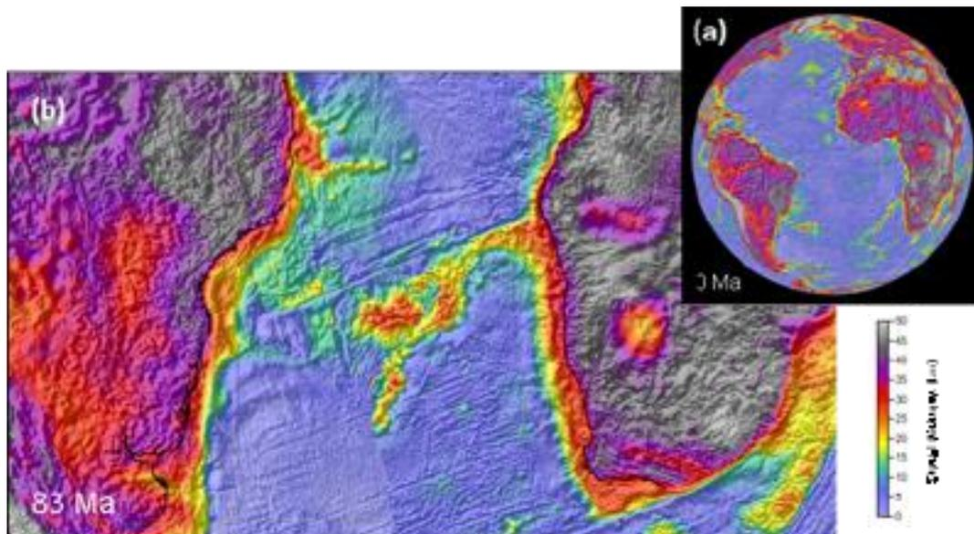
Figure 2 (a) Present day crustal thickness from gravity inversion for the Atlantic Ocean. (b) Crustal thickness restored to 83 Ma using GPlates 1.5.
