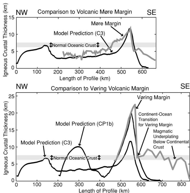
Figure 1: Comparison of numerical modeling results for melt production at the Møre and Vøring margins with observed crustal thicknesses [from Simon *et al.*, 2009].
