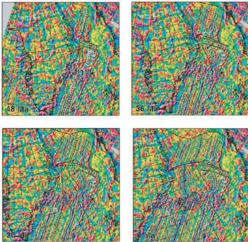
Figure 4. NE Atlantic and Norwegian-Greenland Sea reconstruction of gridded magnetic data (Verhoef et al., 1996), applying the method of Verhoef et al. (1990). Reconstructed grid node positions were achieved by rotating the grids according to plate reconstruction parameters (Müller et al., 1997). The Euler poles are listed in Table 1. These images were extracted from an animation by Lundin et al. (2002). Click on image to enlarge.
